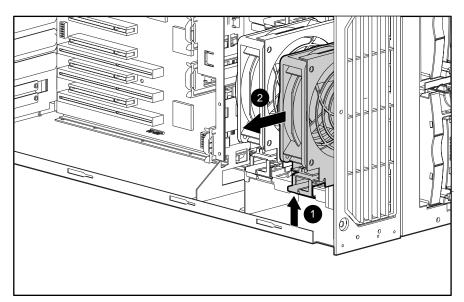
Figure 2-12. Removing a front fan
